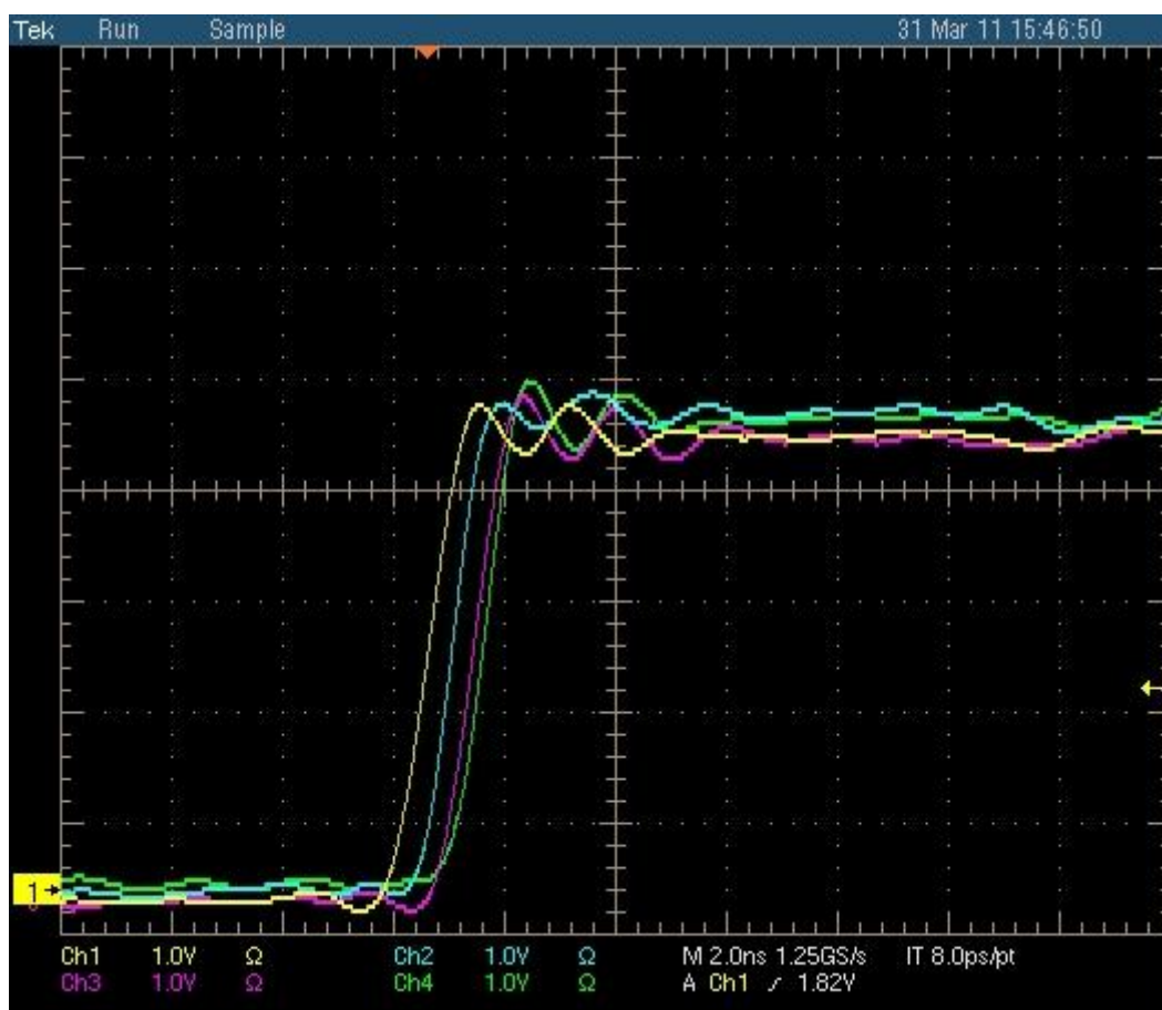
Typical risetime and distribution of the PPS outputs with 2ns/div horizontal scale
